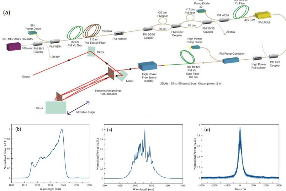
**Fig. 1** (a) 1.5-GHz intra-burst repetition rate Yb-doped all-PM-fiber laser system setup. (b) The oscillator spectrum. Compressor output (c) spectrum and (d) pulse duration for 1  $\mu$ J individual pulse energy, 80-pulse bursts at 25 kHz.
