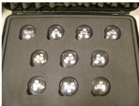
Figure 1. Each material has three samples with different thicknesses in order to study incremental absorption effect in spectral signature.
