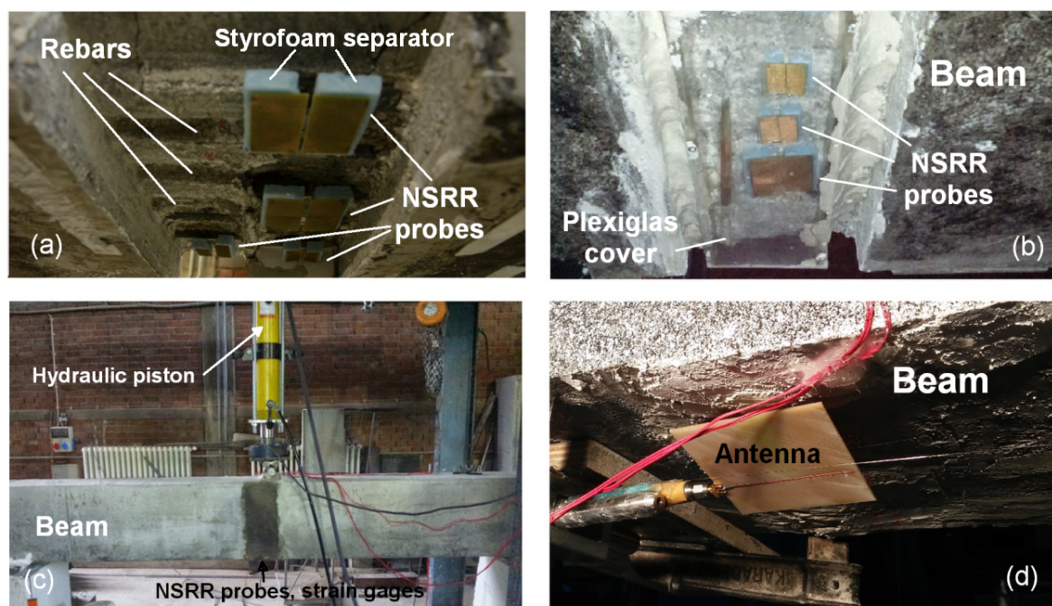
Fig. 3. Preparation of the final experiment setup: a) The arrangement of the NSRR sensors, b) Placement of the protective plexiglas cover, c) The final simply supported beam experiment setup, d) Antenna monitoring the sensors from outside the bottom of the beam.
