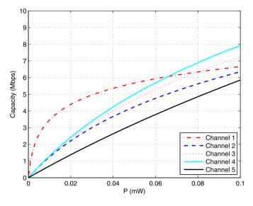
**Fig. 2.** Capacity of each link versus power for the communication between the transmitter and the primary receiver, where  $B_1 = 1$  MHz,  $B_2 = 3$  MHz,  $B_3 = 4$  MHz,  $B_4 = 5$  MHz,  $B_5 = 10$  MHz,  $N_1 = N_2 = N_3 = N_4 = N_5 = 10^{-12}$  W/Hz,  $|h_1^p|^2 = 1$ ,  $|h_2^p|^2 = 0.1$ ,  $|h_3^p|^2 = 0.1$ ,  $|h_4^p|^2 = 0.1$ , and  $|h_5^p|^2 = 0.05$ .
