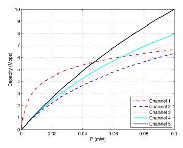
**Fig. 3.** Capacity of each link versus power for the communication between the transmitter and the secondary receiver, where  $B_1 = 1$  MHz,  $B_2 = 3$  MHz,  $B_3 = 4$  MHz,  $B_4 = 5$  MHz,  $B_5 = 10$  MHz,  $N_1 = N_2 = N_3 = N_4 = N_5 = 10^{-12}$  W/Hz,  $|h_1^s|^2 = 1$ ,  $|h_2^s|^2 = 0.1$ ,  $|h_3^s|^2 = 0.1$ ,  $|h_3^s|^2 = 0.1$ , and  $|h_5^s|^2 = 0.1$ .
