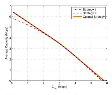
**Fig. 5.** Average capacity versus minimum average capacity requirement for Strategy 1, Strategy 2, and the optimal channel switching strategy for the scenario in Fig. 2 and Fig. 3, where  $P_{av} = 0.05$  mW.
