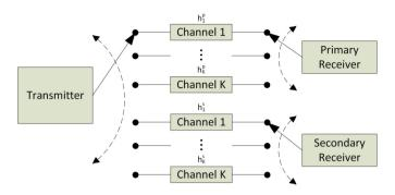
**Fig. 1.** Block diagram of a communication system in which transmitter communicates with primary and secondary receivers via channel switching among K channels (frequency bands). It is noted that the channel coefficients can be different for the same channels.
