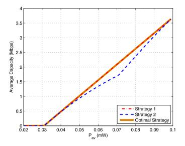
**Fig. 4.** Average capacity versus average power limit for Strategy 1, Strategy 2, and the optimal channel switching strategy for the scenario in Fig. 2 and Fig. 3, where  $C_{\text{req}} = 5$  Mbps.
