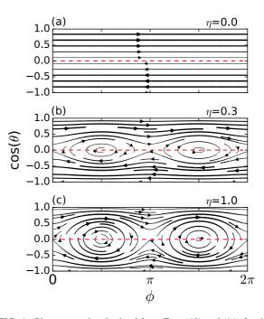
FIG. 1. Phase portraits obtained from Eqs. (10) and (11) for three different  $\eta$  values. Dashed red lines mark the equator on the Bloch sphere. The thickness of the lines is proportional to the speed of the flows.
