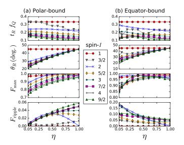
FIG. 3. Rotation instants and angles (in degrees) for the optimal cat-state generation and stabilization as quantified by maximum fidelity  $F_{\text{max}}$  [Eq. (12)] and its ripple  $F_{\text{ripple}}$  [Eq. (13)] for polar-and equator-bound cases.
