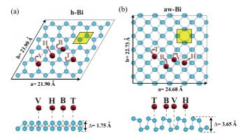
FIG. 3. (a) Description of possible adsorption sites, T, H, B, and V, on the  $(5 \times 5)$  supercells of SL h-Bi in top and side view. Primitive unit cells are shaded. Lattice constants of the supercell and  $\Delta$  buckling parameters are also shown. (b) Same for SL aw-Bi.
