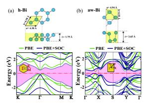
FIG. 1. (a) Top and side views of the unit cell of SL h-Bi with optimized lattice constants and buckling  $\Delta$ . Electronic energy band structures of bare SL h-Bi structure calculated using PBE, PBE+SOC. Zero of band energy is taken at the top of the valence band. (b) Same for SL aw-Bi.
