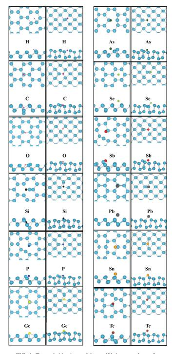
FIG. 4. Top and side views of the equilibrium atomic configuration of adatoms adsorbed to SL h-Bi (first and third columns) and SL aw-Bi (second and fourth columns). Host Bi atoms are shown by large, turquoise balls.
