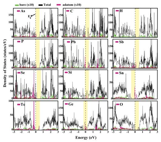
FIG. 5. Total density of states (TDOS) calculated for a single adatom adsorbed to each  $(5 \times 5)$  supercell of h-Bi at the corresponding equilibrium site is shown by thin black lines. The density of states of the "bare" extended h-Bi substrate is shown by a light blue tone; its band gap is shaded by a yellow zone. Pink lines indicate TDOS projected onto the adatom. The zero of the energy is set at the common Fermi level shown by a dashed vertical line.
