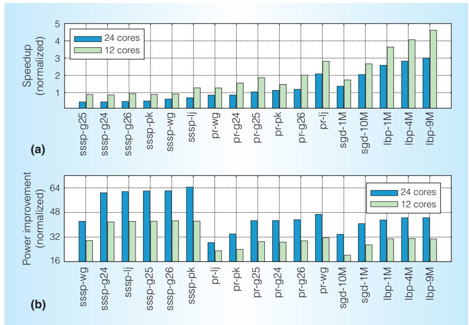
Figure 3. Power and performance comparison of the accelerator (ACC) and CPU. The y-axis is the speedup and power improvement of the proposed accelerator normalized with respect to accelerator execution. (a) Execution time. (b) Power consumption.
