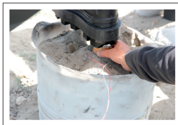
Figure 6. Explosive placement before the blast tests.
