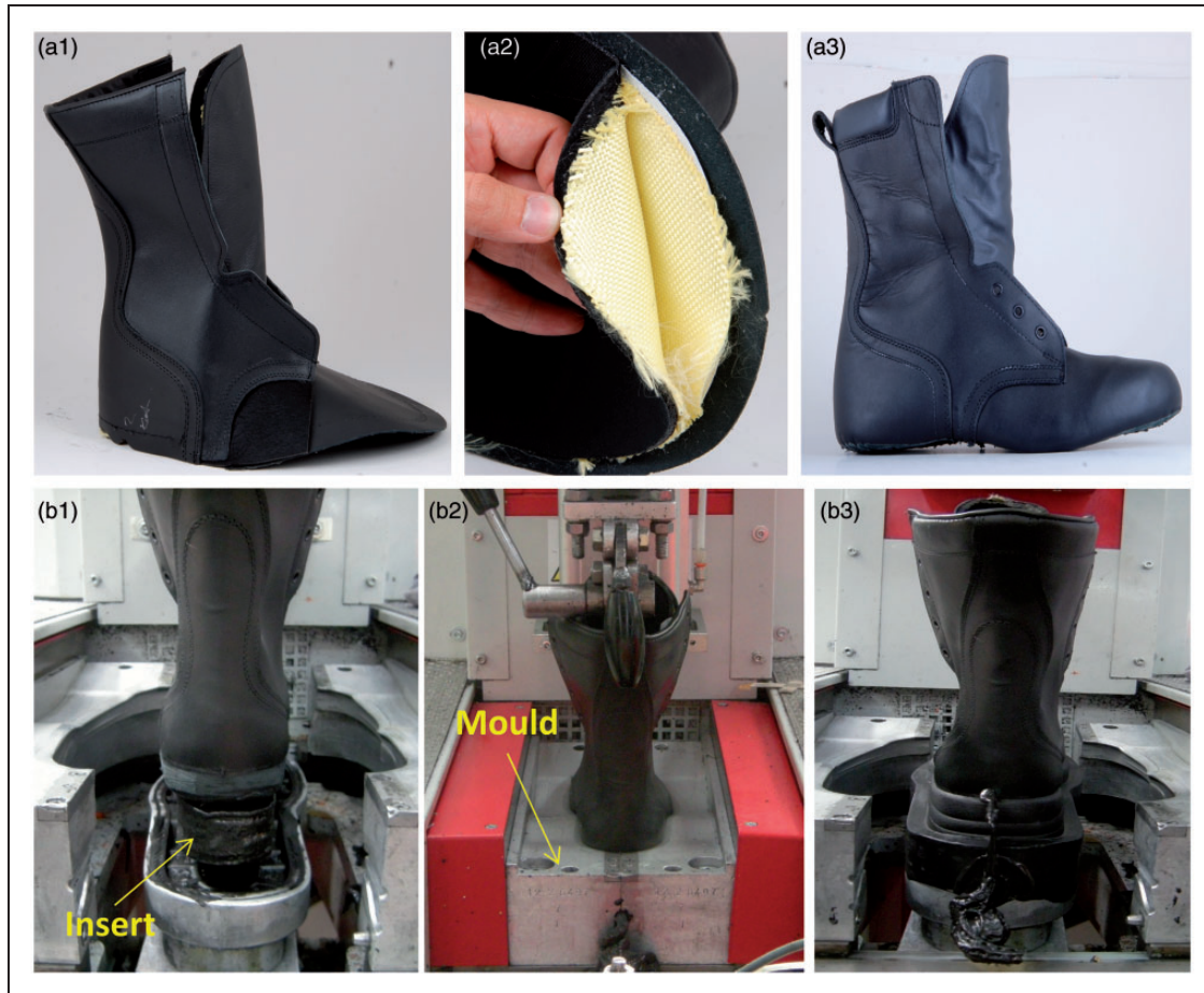
Figure 3. Manufacturing steps of the boots: (a) the vamp and (b) the rubber injection process.
