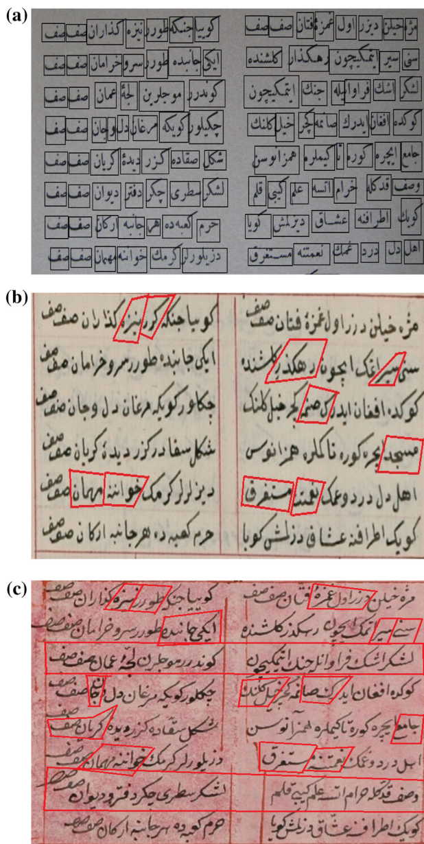
Fig. 11 First image is used a printed version of a poem, while second and third ones are handwritten versions which are from sixteenth century. Manually segmented words in printed version are used as query words to segment second version and these automatically extracted words in second version are used query words to segment third version into words this time. Mismatches are showed in boxes and reason for this is the connected sub-words and writing variations in different versions
