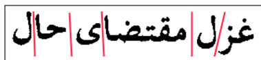
Fig. 3 All the black pixel groups are individual connected components (CC). There are 11 CCs in this image (six of them are major, and five of them are minor) that are merged to result in six sub-words. Sub-words are separated by lines
