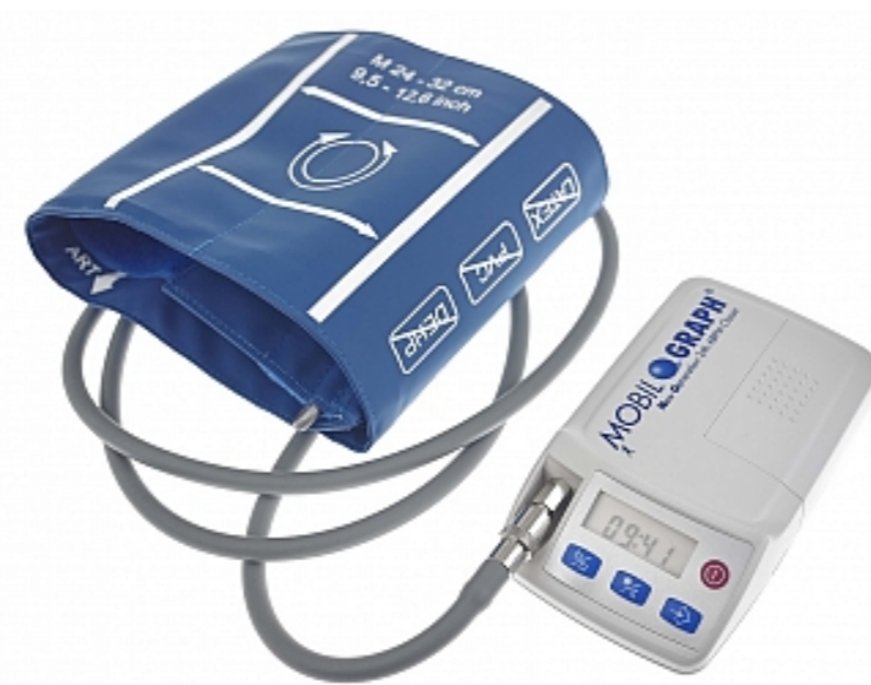
Fig. 2: Mobil-O-Graph for measurements of arterial pressure and pulse wave form
