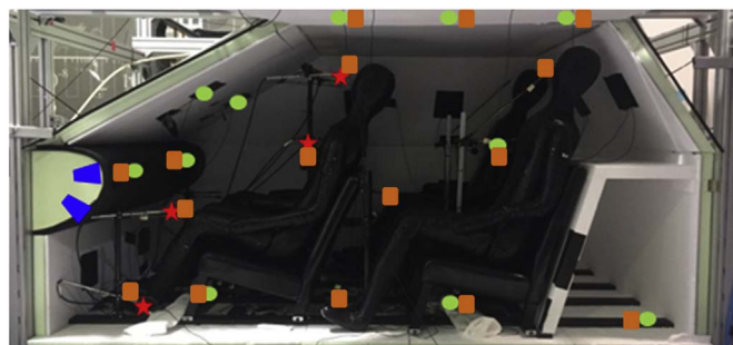
★ Omnidirectional velocity and temperature probes ● Resistance temperature detectors ■ Infrared camera ■ Humidity Sensors
