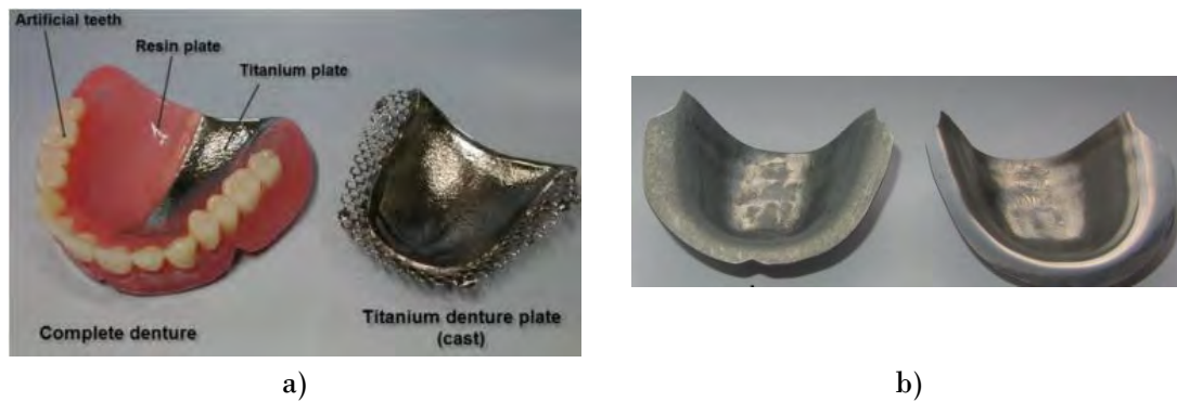
Figure 2.46. a) Complete cast-metal denture base and b) SPIF manufactured denture base in DC04 (left) and X6Cr17 (right) (Milutinovic et al., 2014).
