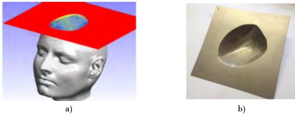
Figure 2.52. Skull model (a) and finished part (b) (Lu et al., 2016).
