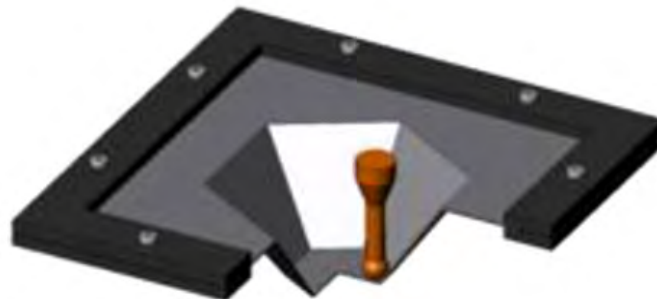
Figure 2.2. SPIF variant (Allwood et al., 2010).
