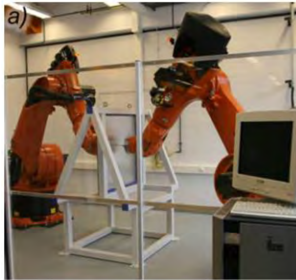
Figure 2.14. Experimental set-up of Roboforming (Meier et al., 2009).
