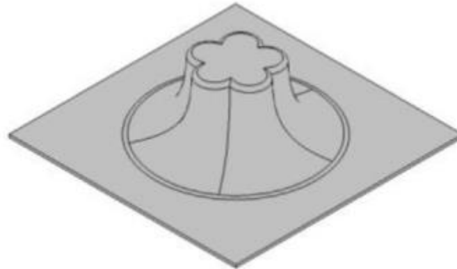
Figure 2.31. Variable wall angle truncated lobe conical geometry proposed to determine SFFL (Soeiro et al., 2015).
