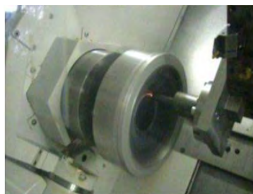
Figure 2.11. High-speed SPiF in a CNC lathe (Ambrogio et al., 2013).
