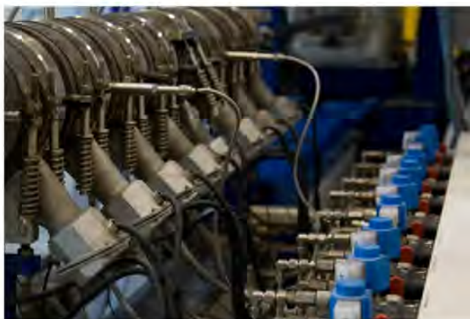
110 Fig. 1. Photograph of the Cleextral (France) Evolum HT 53 co-penetrating and co-rotating twin- 111 screw extruder used for the thermo-mechanical fractionation of rice straw biomass (53 mm for the 112 D screw diameter, 36D for the total barrel length).
