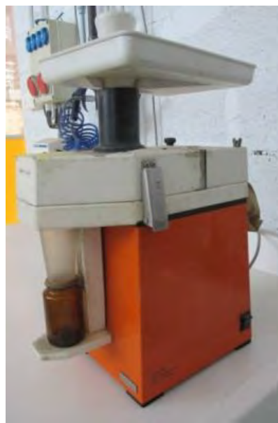
Figure 5. Foss mill, Cyclotec 1093, Denmark.
