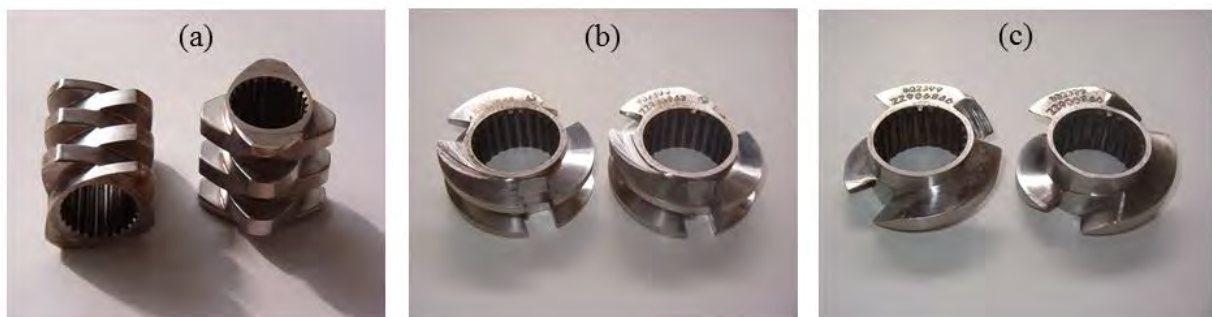
Figure 10. Segmental screw elements: BL22-90° bilobe paddle-screws (a), reversed simple-thread (b), and conveying simple-thread screws (c).
