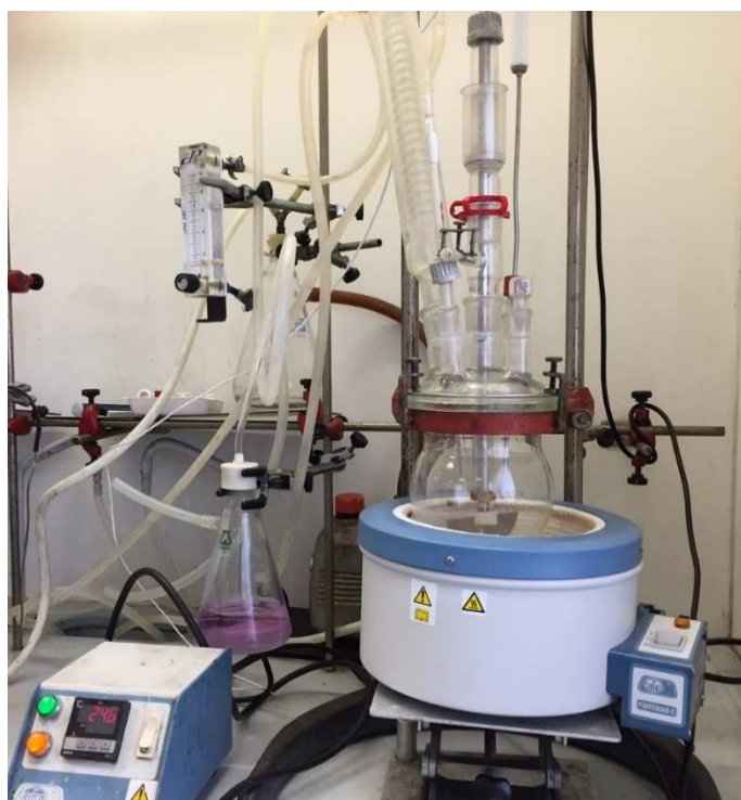
Figure 3.3 Real reaction assembly used for carbodiimide synthesis.
