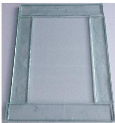
Figure 3.4 Mold used to prepare polyurethane films
