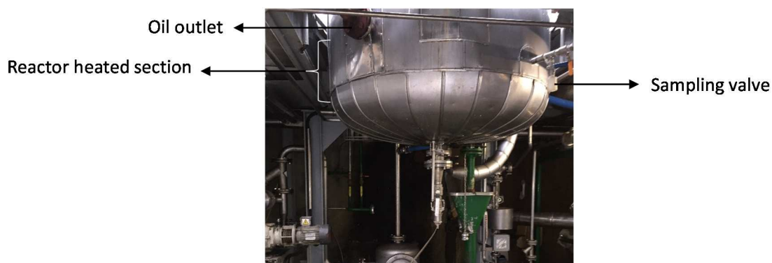
Figure 7.6 Bottom of the 1 m 3 reactor used.
