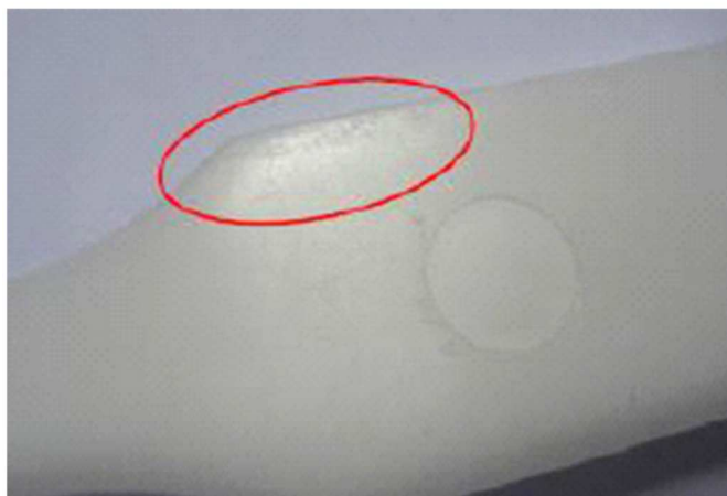
Figure 6.15 Amplified picture of the polypropylene reference specimen after the climate cycles test exposition.
