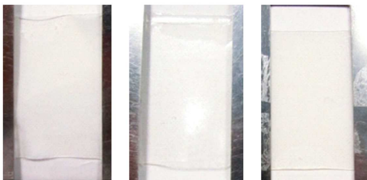
Figure 6.4 PU with 5% of CDI R11, before and after 200 h subjected to external ageing test.
