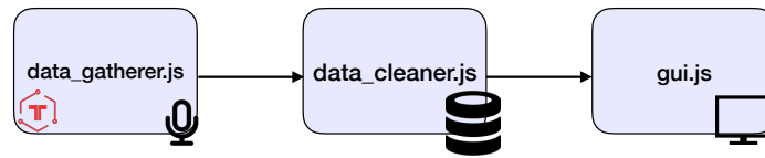
Figure 6.6. Topology implemented during the Software Atelier 3 project
