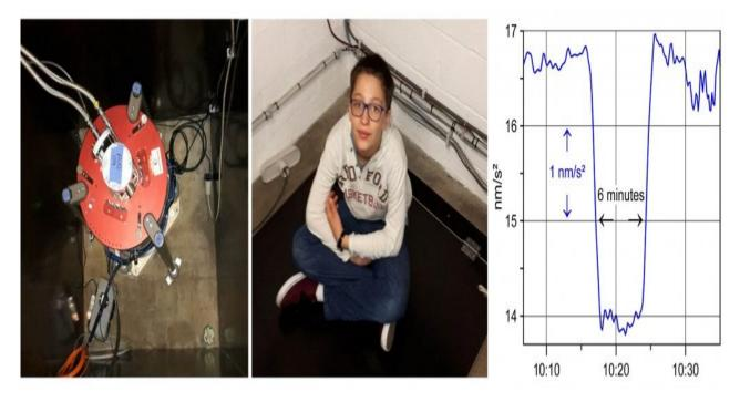
Left: A superconducting gravimeter installed in a shaft at the Rochefort station, Belgium. Center: A 13-year old boy, weighing 45 kilograms, sat with his navel 1 meter above the instrument. Right: The gravitational effect of the boy sitting for 6 minutes: his mass induced a decrease in gravity of 0.28 billionth of g. Credit: Royal Observatory of Belgium/Van Camp et al, 2017 (http://onlinelibrary.wiley.com/doi/10.1002/2017RG000566/full), Figures A4d and A7
