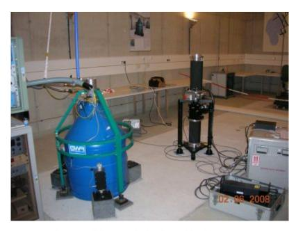
Superconducting (blue) and absolute (black) gravimeters measuring at Conrad Observatory, Austria. Credit: Olivier Francis
