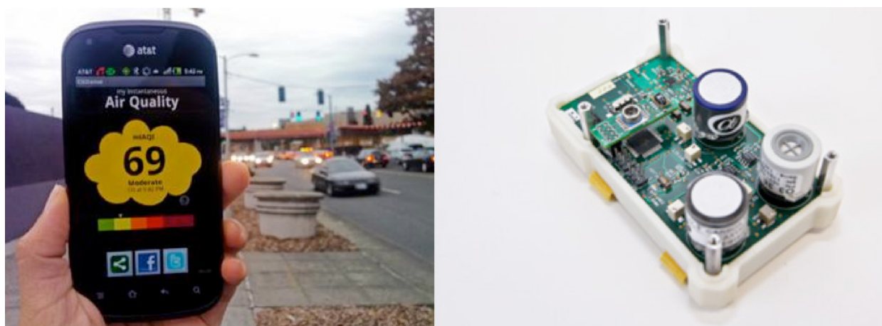
Figure 3. The CitiSense mobile app (left) and a view of the inside of the CitiSense sensor (right). Photo credit: http://www.calit2.net/ .
