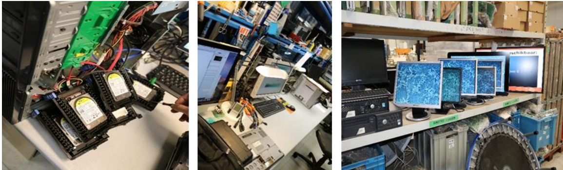
Figure 3 — Data deletion system, repair workbench and testing station for reused and repaired electronics at De Kringwinkel Hageland.
