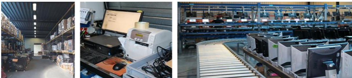
Figure 4 — Warehouse, unloading workstation and transportation system for products to the other workstations for repair and refurbishing.
