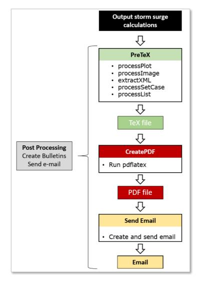
Figure 6 - Procedures for the SSCS bulletins
