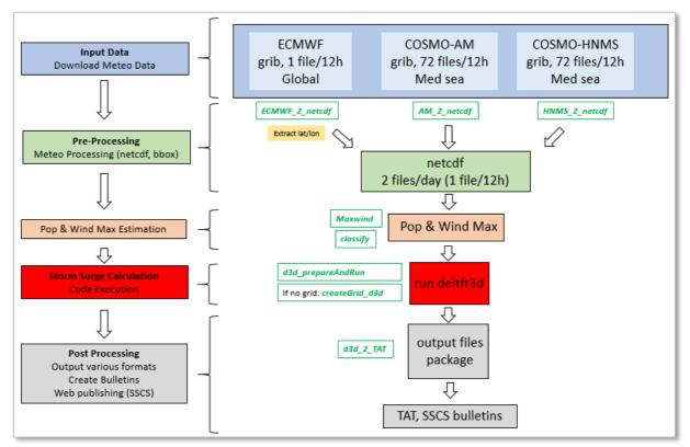
Figure 4 – SSCS-Delft3D Procedure.
