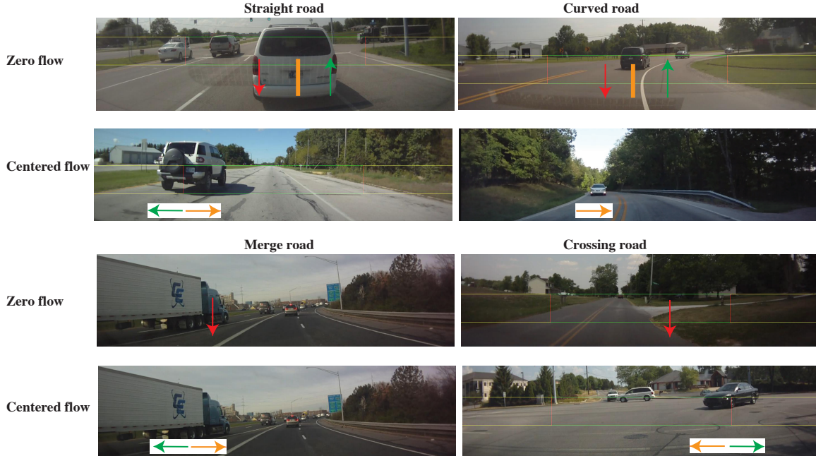
Fig. 6. Different road collision cases cause horizontal motion and vertical flow expansion. The red arrows indicate motion direction of potential collision, green arrows mean safe motion, and orange arrows mean centered motion direction required attention. The vehicle heading direction is at the image center.
