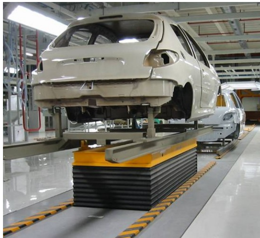
Figure 3.10. A skillet conveyor holding a chassis. (ASAS, 2018)
