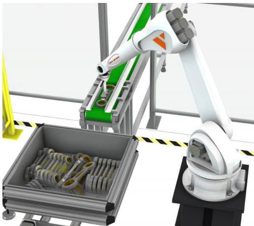
Figure 2.1. In addition to discrete-event simulation, continuous simulation with physics engine can be utilized, for example, in bin picking process
