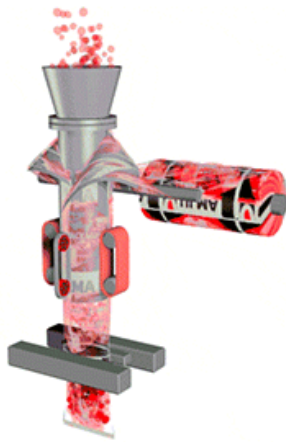
Figure 3.15. The principle of vertical form-fill-seal process. (ULMA Vertical, 2018)
