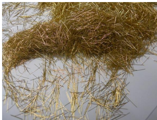
Figure 16 Copper coated steel fibers used for producing UHPFRC (Aspect ratio=65).
