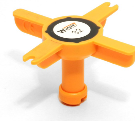
Figure 43 An older SolidRH SH1 sensor that requires a separate RD1 reading device (Wiiste 2015)
