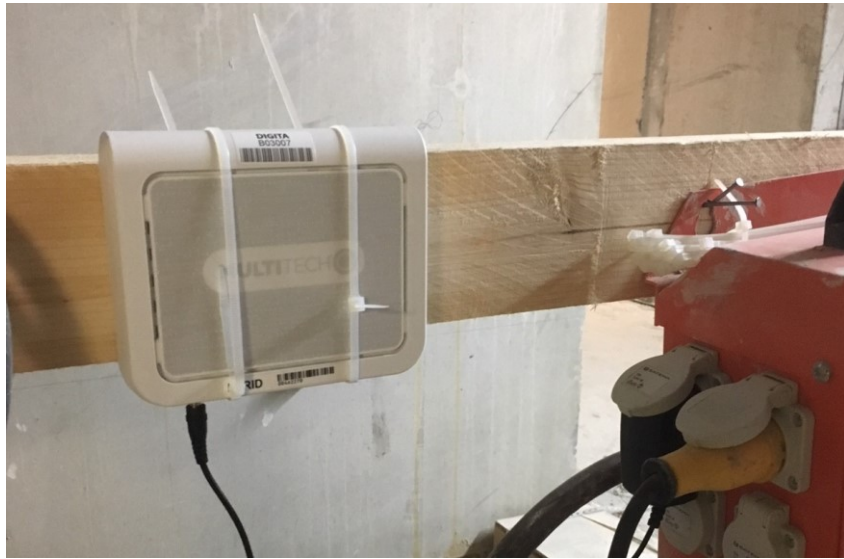
Figure 63 A LoRaWAN base station is sometimes required if the transmission range is not satisfactory
