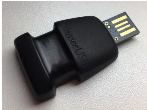
Figure 46 Thingsee sink is very compact and is connected directly into an USB port
