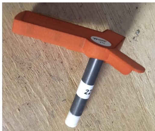
Figure 44 A prototype of the upcoming LoRaWAN-sensor, the casing is 3D printed
