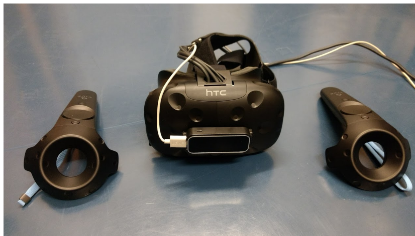
Figure 3.1: An photograph of the HTC Vive head-mounted display and the attached Leap Motion hand-tracking device, and the Vive Wand hand controllers.
