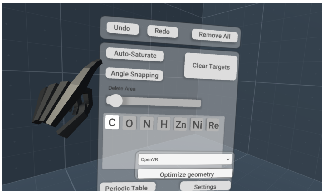
Figure 5.4: Picture of the floating menu used with Leap Motion hand tracking. The buttons are activated by touching them with the virtual hands, but the lack of physical feedback often makes this difficult.
