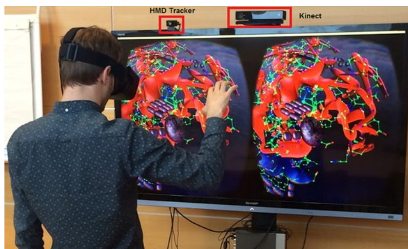
Figure 2.5: Image of the Molecular Rift setup and a mirrored image of the view inside the HMD.
