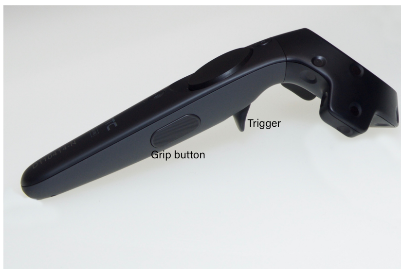
Figure 5.3: Picture of a HTC Vive Wand controller with labels for the buttons primarily used in VRChem.
