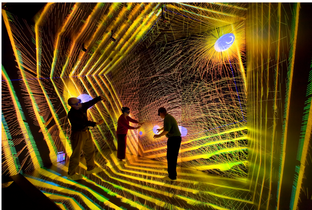
Figure 2.3: A CAVE virtual reality system displaying an astronomical simulation.
