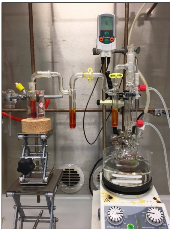
Image 3: Photo of the apparatus used for the methoxyl group determination
