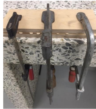
Figure 24 - Cold pressing using screw clamps.
