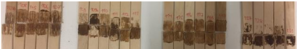
Figure 35- Types of bond failure occurring in different samples. From left to right: Gelatin + CLP (HP), gelatin + CLP (CP), gelatin + ESL (HP) & gelatin + ESL (CP)
