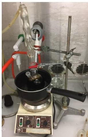
Figure 15 - The equipment for cationic lignin preparation.
