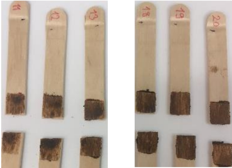
Figure 34 a-b – Broken bonds of hot-pressed Lignoboost (11-13) & CLPs (18-20).
