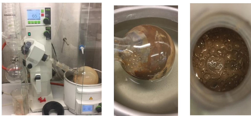
Figure 17a-c - CLP concentration with rotavapor.
