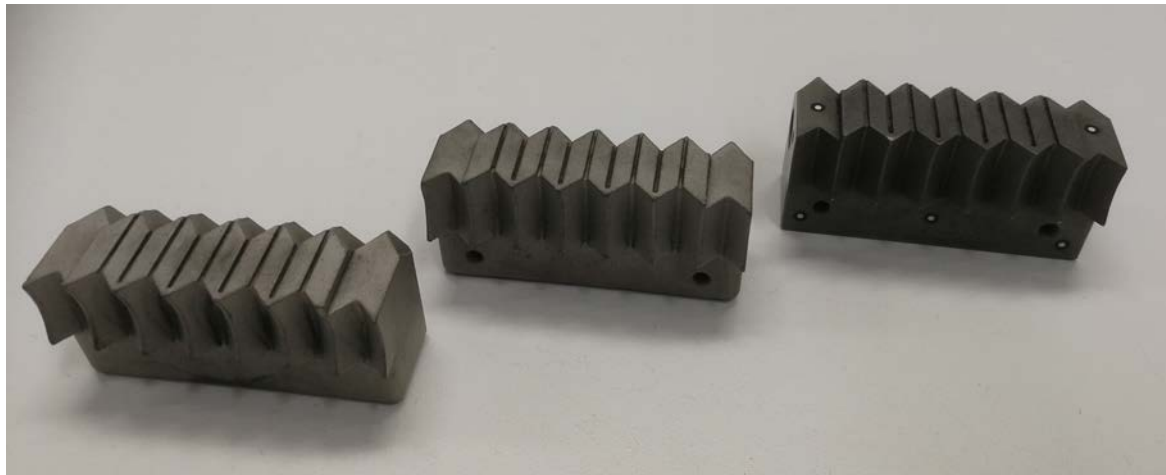
Figure 9. Heated cutter at different stages of precision casting: On the left, the cast piece; in the centre, the machined piece; and on the right, the machined and tempered piece.
