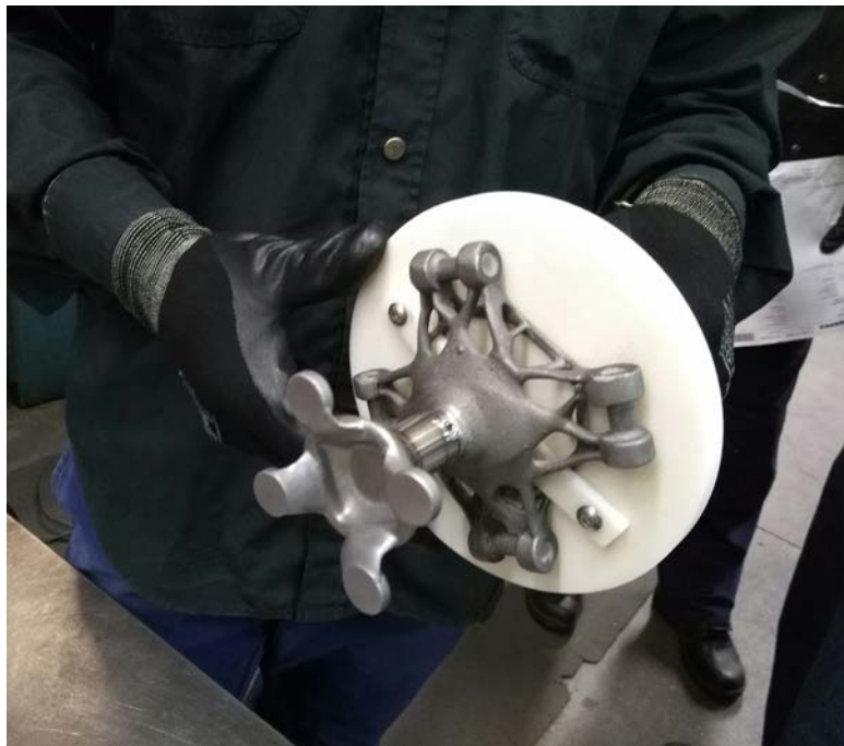
Figure 19. The blade hub after laser welding.
