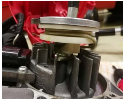
Figure 21. 3D printed gear after installation.
