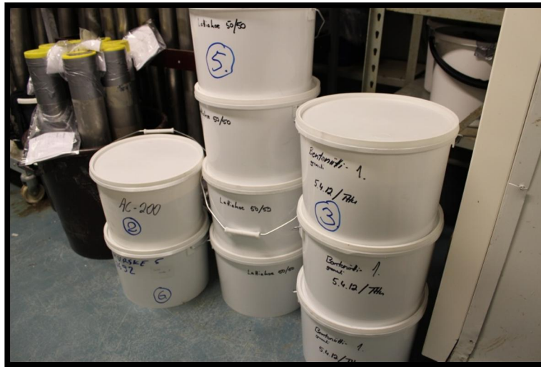
Figure 4-1. Granular materials are stored in air-tight buckets inside the cold room.
