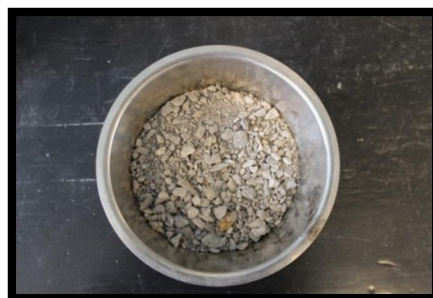
Foundation bed mixture
