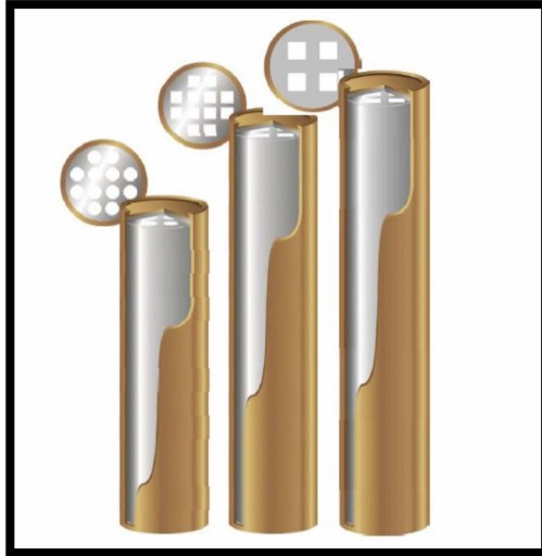
Figure 2-6. Different kinds of disposal canisters for spent fuel with both containers (Posiva 2010, p.25).
