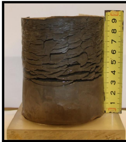
Figure 6-19. Picture of the frozen sample after the freezing-thawing test (Initial height 100mm)
