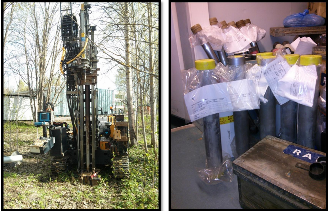
Figure 6-9. Pictures of the sampling process (left) and the storage (right) of the sampler tubes in the cold room (average temperature +7^{\circ}\text{C} )
