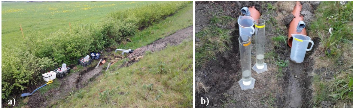
Figure 14. a) Data gathering in progress on June 8, 2017. b) 3-litre cans were used for sample gathering, and 1000-ml measuring glasses for manual flow rate measurements.
