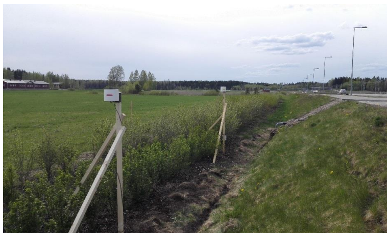
Figure 13. Rain gauges at the test site used for continuous precipitation monitoring.
