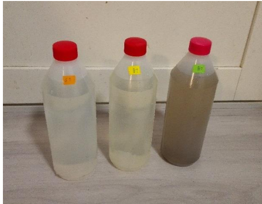
Figure 31. Color of the filter effluents and untreated stormwater. Sampled waters in 1-liter bottles from the sand filter (left), the sand-biochar filter (middle) and the untreated stormwater (right). The effluent from the sand filter was the most transparent and colorless, while the effluent from the sand-biochar filter was slightly yellowish and stormwater dark grey. The colors were similar throughout the study, although the shades varied.
