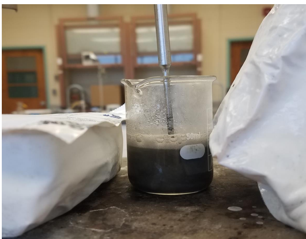
Figure 1: Experimental setup to magnetic stir and tip sonicate solution at the same time
