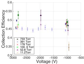
**FIGURE 2.** *Left*: The radon emanation measurement system at SDSM&T – components and operation described in text. *Right*: The efficiency for collecting radon daughters onto the silicon-pin diode in a nitrogen atmosphere does not vary significantly with changes in voltage or pressure. Lighter points correspond to collection efficiency for <sup>218</sup>Po, while the darker points are for <sup>214</sup>Po. SDSM&T operates at around 100 Torr and -2000 V.
