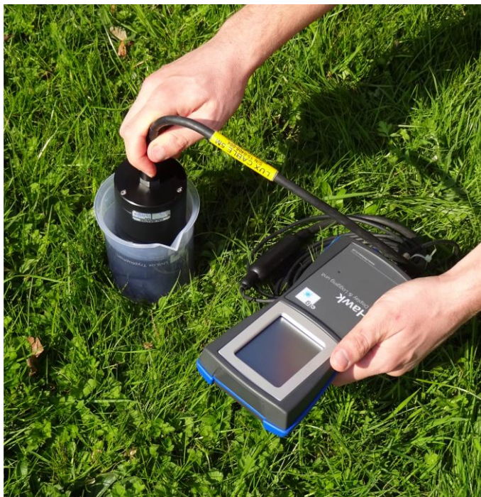
Figure 7. Instantaneous assessment of faecal contamination in drinking water using a tryptophan-like fluorimeter in a beaker and a handheld reader. Note that the sensor operates using UV light and is sensitive to sunlight; hence, the beaker would need to be covered for a reliable measurement.
