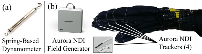
Figure 4 – Experimental setup for tendon pre-loading tests: (a) the dynamometer used for tendon tension measurements. (b) Magnetic trackers and field generator Aurora NDI system for fingertip, PIP, DIP and MCP trajectory data acquisition.
