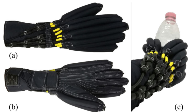
Figure 1 - Overview of the AirExGlove: (a) hand dorsal side of the system (pneumatic chambers pressurized), (b) hand palm side (tendon channel seams visible in white) and (c) side view of the system (thumb side) when grasping a plastic bottle.
