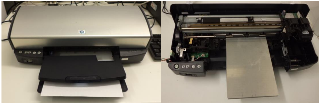
547 Figure 1: Image of out-of-the-box HP 5940 printer (left) and modified printer with stationary stage positioned 548 (right)
