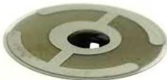
Figure 77: The crude-GCM composite resonator shown here before heating to disperse the heavy crude.
