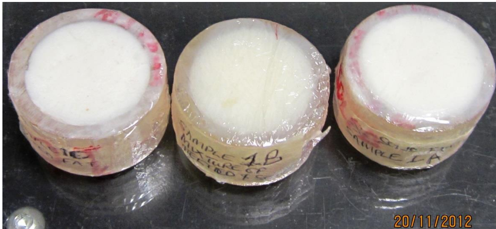
Figure 3.2: single tissue phantoms containing lard. These were used to test the suitability of using lard to create fat nodules in the two-tissue phantoms.
