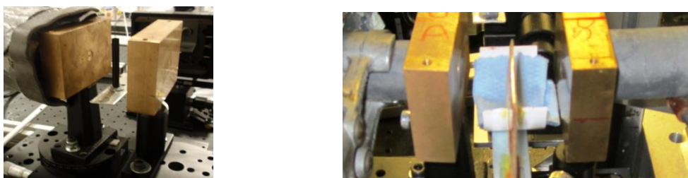
Figure 3.3: Photographs showing the arrangement of the diffraction cell. The non-parallel arrangement of the two collimator blocks (SC & DC) ensures a scattering angle of six degrees. In the RH image the caffeine test sample can be seen mounted on the horizontal translation slide.
