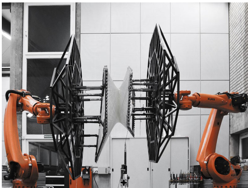
Figure 55: ICD/ ITKE Research Pavilion 2012, robotic manufacturing.
