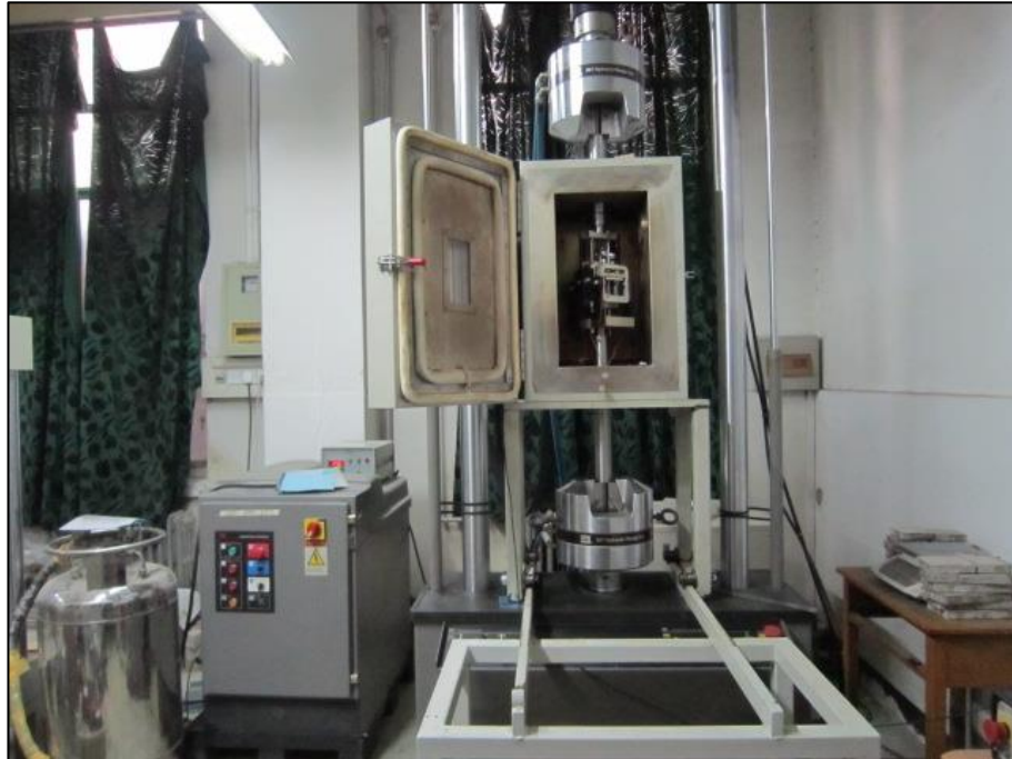
Fig 3.15 The 4PB apparatus in an environmental chamber on the MTS
