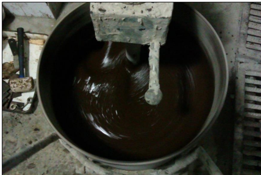
Fig 3.5 The CAM mixing in a 2.5-Litre stirring mixer
