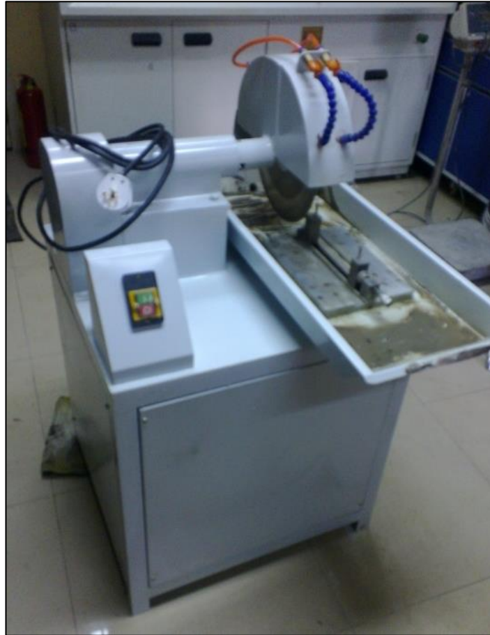
Fig 3.7 A cutting machine for mortar and concrete
