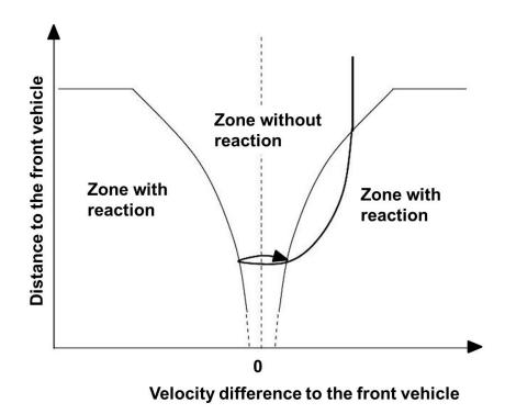
Figure 2.1: An example of perception threshold of the psycho-physical model (Source: Olstam and Tapani, 2004 [13])
