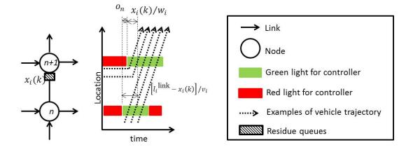
Figure 3.6: Offset control with residue queues
