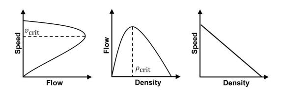
Figure 2.2: Fundamental diagrams
