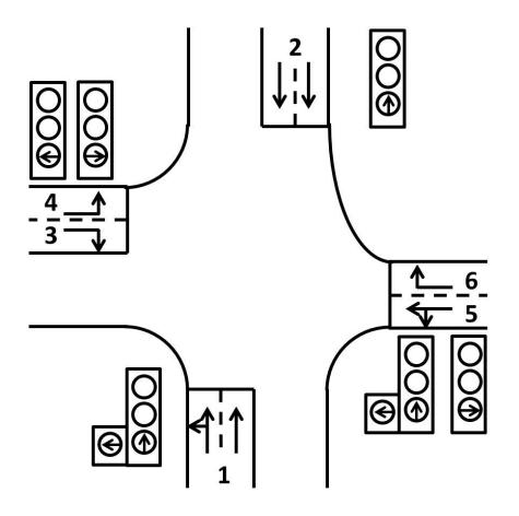
Figure 2.3: Different phases of a signalised intersection
