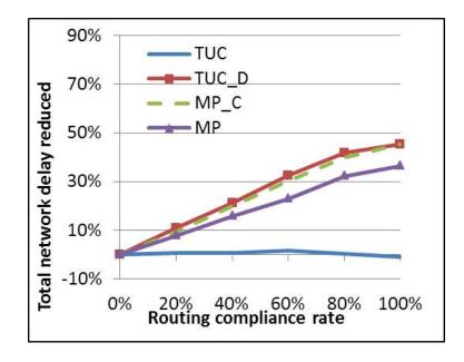
Figure 5.27: Average network delay of the three by three grid network over different rerouting compliance rate  $\sigma = 0.9$
