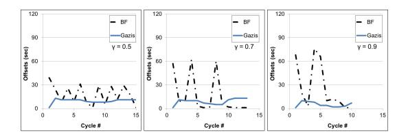
Figure 4.9: Offsets at Node 3 over different  $\gamma$  on the two-way arterial network
