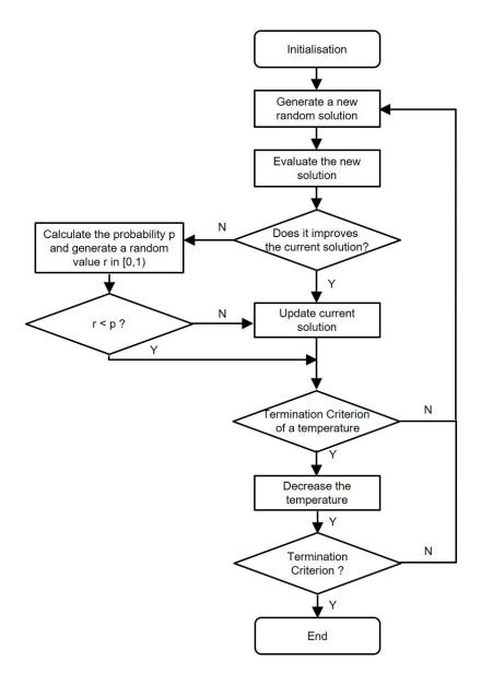
Figure 2.12: A flowchart of Simulated Annealing
