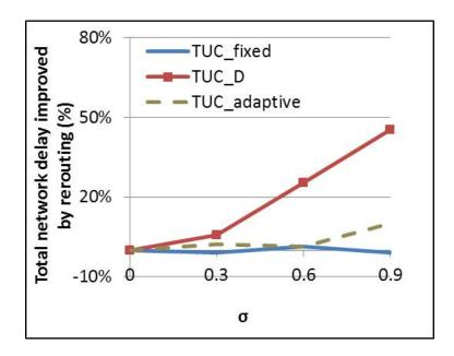
Figure 5.43: Improvement of network delay by rerouting over  $\sigma$
