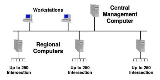
Figure 2.6: Architecture of a SCATS system
