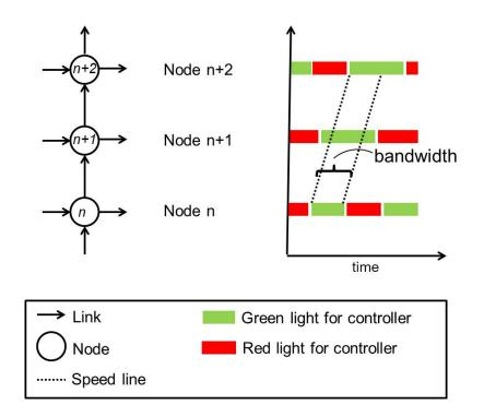
Figure 5.9: An example of a green band formed on an arterial network
