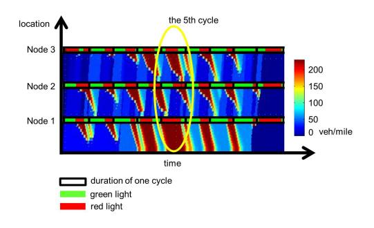
Figure 4.5: Density plot at  $\gamma = 0.9$  on the one-way arterial network controlled by the brute force approach
