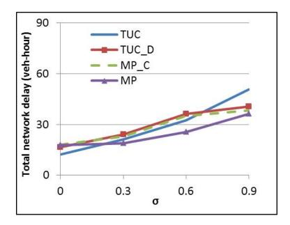
Figure 5.22: Average network delay of the three by three grid network over  $\sigma$  with rerouting
