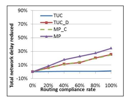
Figure 5.26: Average network delay of the three by three grid network over different rerouting compliance rate  $\sigma = 0.6$
