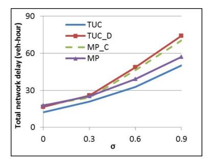
Figure 5.19: Average network delay of the three by three grid network over  $\sigma$  without rerouting
