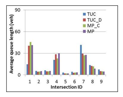
Figure 5.21: Average queue length at intersections of the three by three grid network
