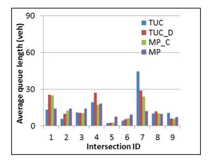
Figure 5.24: Average queue length at intersections of the three by three grid network
