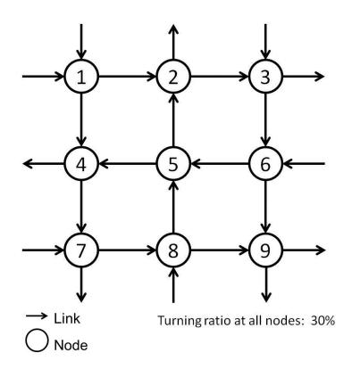
Figure 4.10: Test grid network
