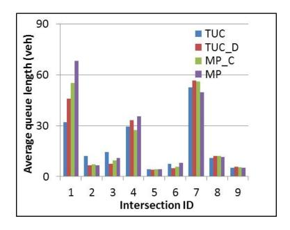
Figure 5.15: Average queue length at intersections of the three by three grid network
