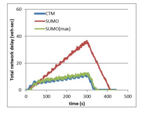
Figure 5.5: Network delay of CTM and SUMO when oversaturated
