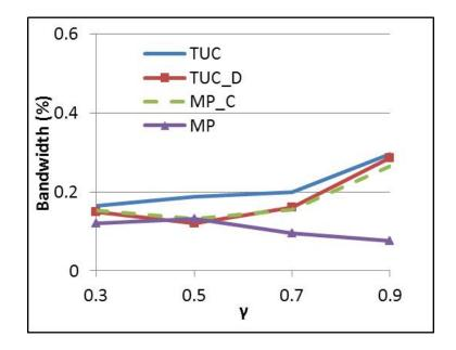
Figure 5.17: Average green bandwidth of the three by three grid network over  $\gamma$  with rerouting
