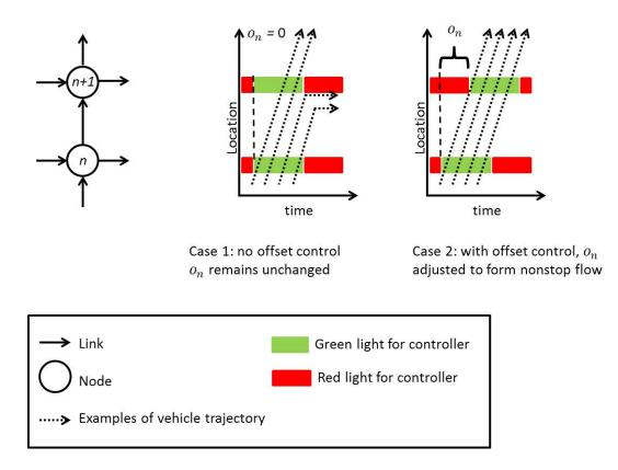
Figure 3.5: An illustration of offset control
