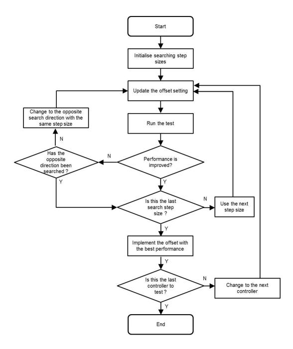
Figure 4.14: A flowchart of hill climbing offset control
