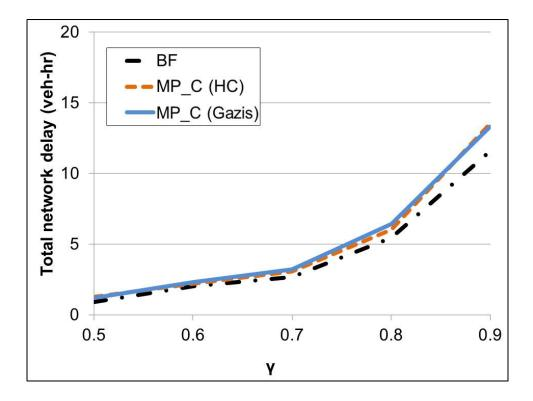
Figure 4.16: Network delays in the one-way arterial network with hill climbing offset controller
