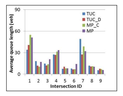
Figure 5.18: Average queue length at intersections of the three by three grid network
