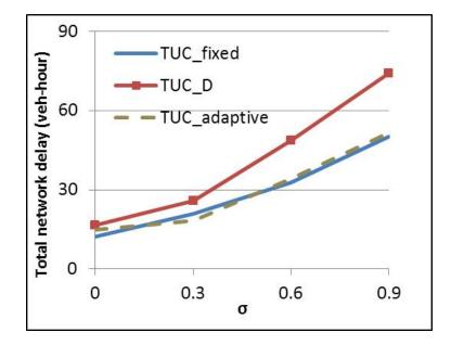
Figure 5.41: Network delay of three TUC systems over  $\sigma$  without rerouting
