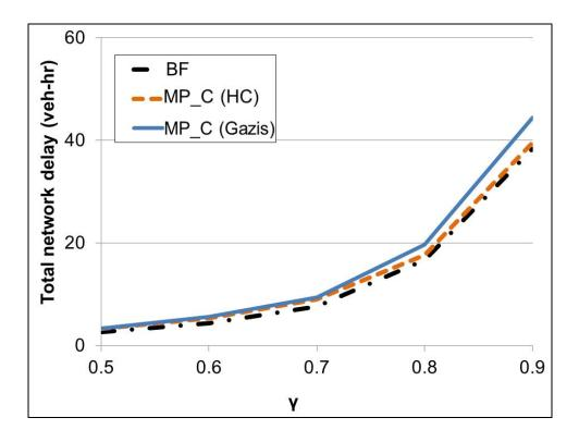
Figure 4.18: Network delays in the grid network with hill climbing offset controller
