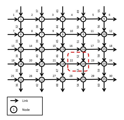
Figure 5.28: Test five by five grid network
