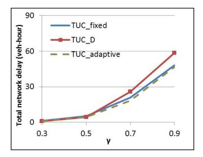
Figure 5.38: Network delay of three TUC systems over  $\gamma$  without rerouting
