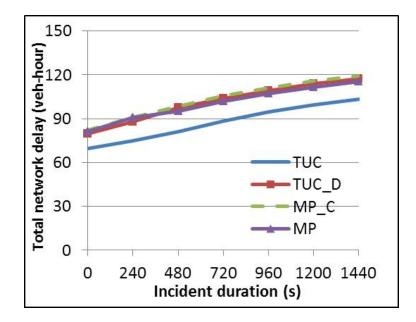
Figure 5.29: Network delay of the road incident scenario without rerouting
