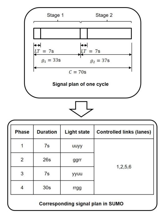
Figure 5.7: An example of the signal plan in SUMO
