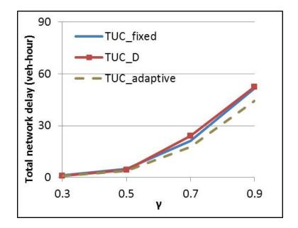
Figure 5.39: Network delay of three TUC systems over  $\gamma$  with rerouting
