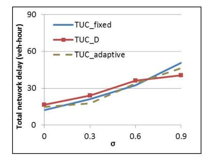
Figure 5.42: Network delay of three TUC systems over  $\sigma$  with rerouting
