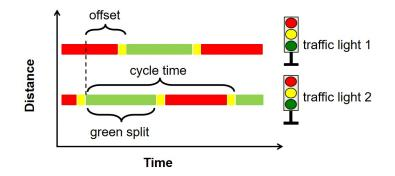
Figure 2.5: An illustration of signal settings
