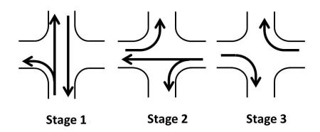
Figure 2.4: Different stages of a signalised intersection
