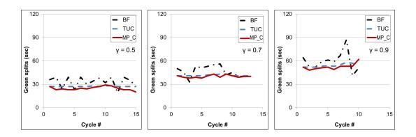
Figure 4.8: Green splits at Node 3 over different  $\gamma$  on the two-way arterial network
