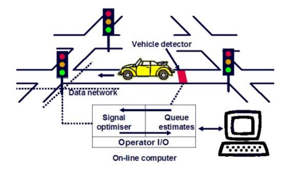
Figure 1.2: An example of urban traffic control system: SCOOT (Source: Peek Traffic Ltd, Siemens PLC and TRL Limited [5])
