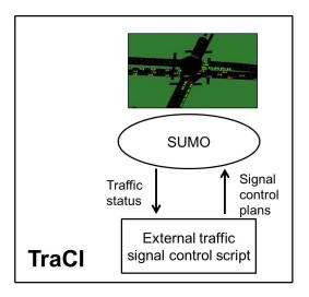
Figure 5.6: Traffic control interface of SUMO
