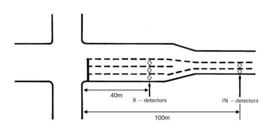
Figure 2.7: Locations of MOVA system's loop detectors
