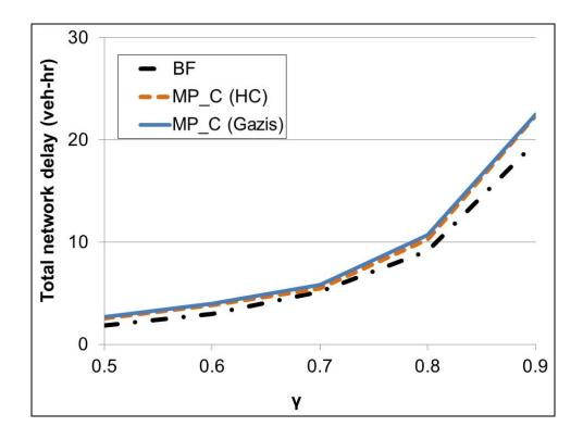
Figure 4.17: Network delays in the two-way arterial network with hill climbing offset controller
