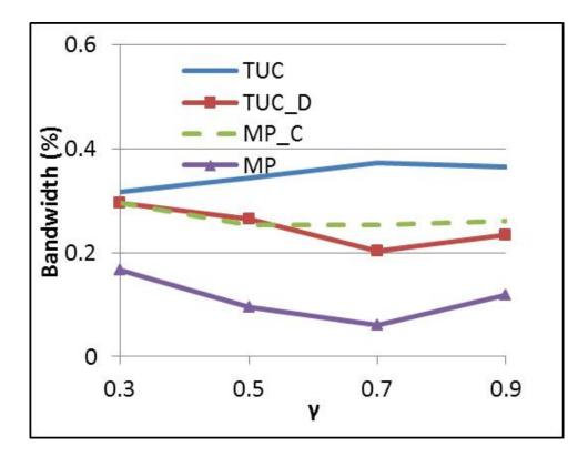
Figure 5.11: Average green bandwidth of the one-way arterial network over  $\gamma$
