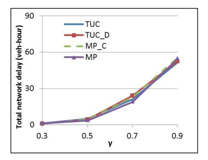
Figure 5.16: Average network delay of the three by three grid network over  $\gamma$  with rerouting
