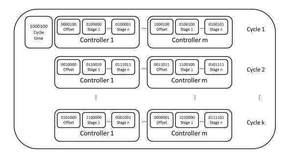
Figure 3.3: A chromosome structure of a network signal plan
