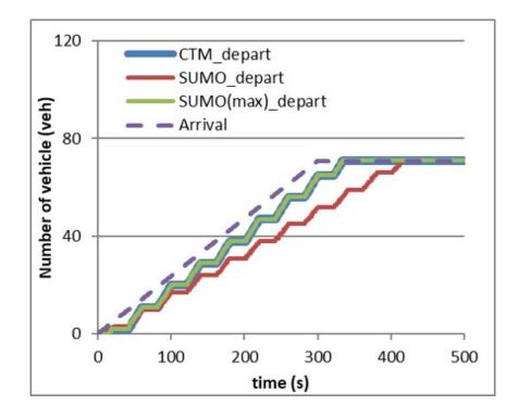
Figure 5.3: Arrival and departure curves of CTM and SUMO when oversaturated
