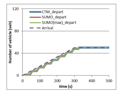
Figure 5.2: Arrival and departure curves of CTM and SUMO when undersaturated
