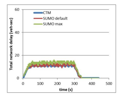
Figure 5.4: Network delay of CTM and SUMO when undersaturated
