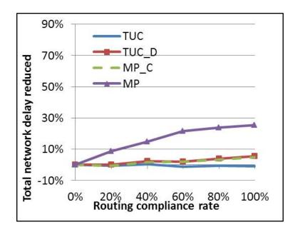
Figure 5.25: Average network delay of the three by three grid network over different rerouting compliance rate  $\sigma = 0.3$
