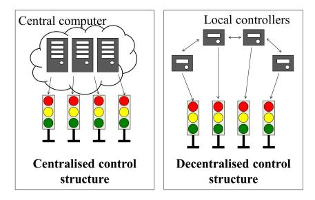
Figure 1.3: Different control structures of traffic control systems
