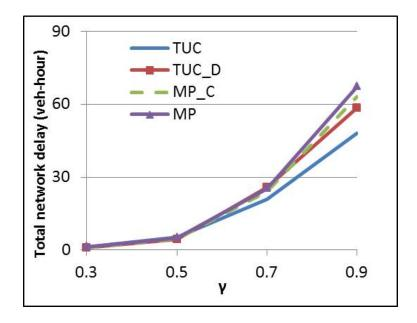
Figure 5.13: Average network delay of the three by three grid network over  $\gamma$  without rerouting
