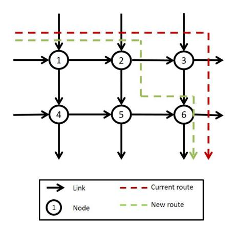
Figure 5.1: An illustration of rerouting on a road network
