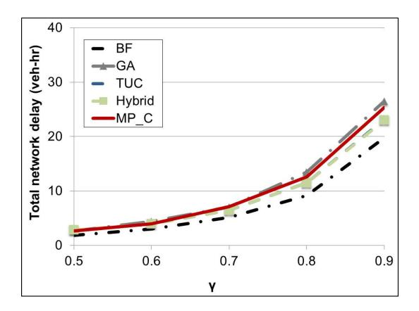
Figure 4.7: Average network delays on the two-way arterial
