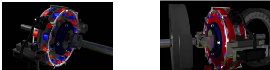
Fig. 13: Developed concept with stator and exploded casing
