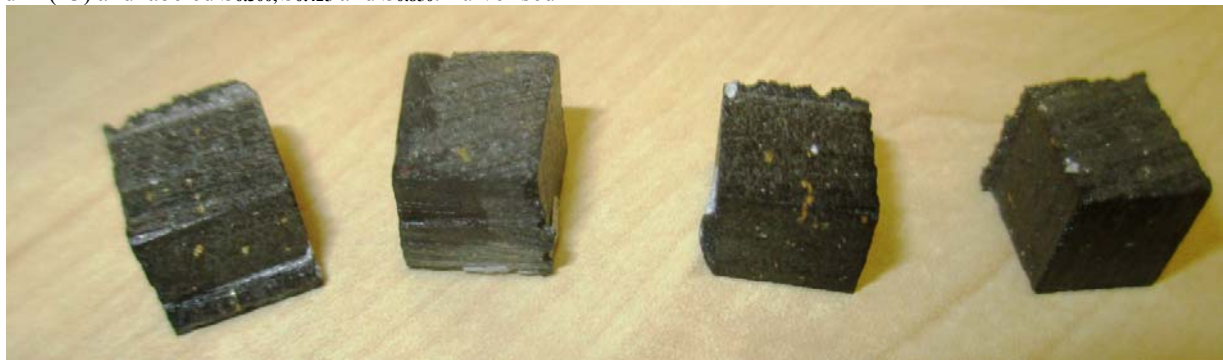
Figure 1: Developed NAO friction lining cut into experimental size of 10 x 10 mm
