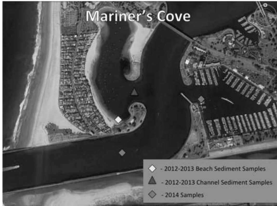
Figure 2.2 Map of Mariner's Cove showing sediment collection sites. The light diamond marks site where beach samples were taken in 2012-2013. The triangle marks where channel samples were taken in 2012-2013. The dark diamonds mark sites where samples were taken in Quivira Basin (right) and Mission Bay channel (center) in 2014.
