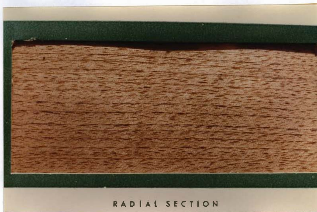
Figure 6. Radial wood section (Harrar, 1967).
