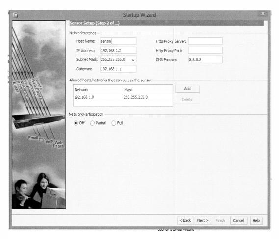
Figure E-3: Showing host name and IP address configuration
