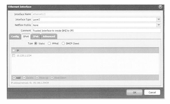
Figure 3.6: Showing IP address configuration on the interface
