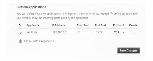
Figure 3.3: Showing configuration to open many ports
