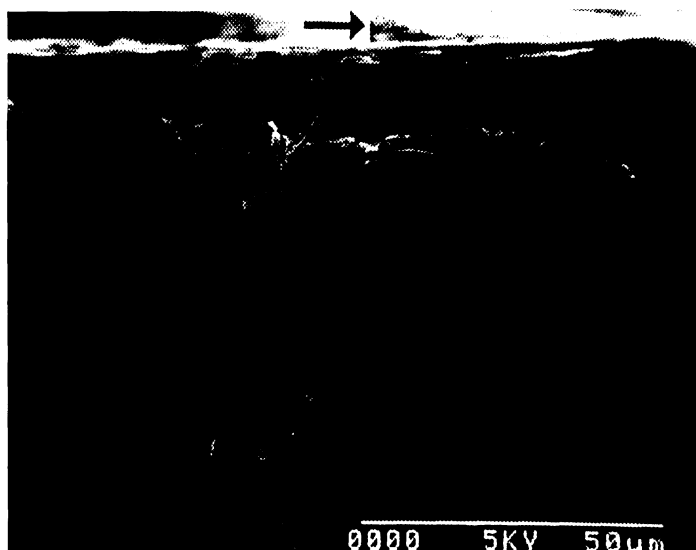
Figure 38. SEM micrograph showed three-layer microstructural feature after lubricated electrical sliding. The Cu matrix was deeply etched. Arrow shows sliding direction.
