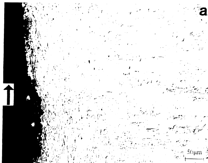
Figure 37. Face section microstructure of the Cu-15vol.%Cr in situ composite, (a) after dry electrical sliding; (b) enlarged view of interfacial microstructure in (a); (c) after lubricated electrical sliding. Arrow shows sliding direction.
