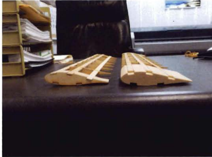
Figure 17: A full size airfoil under construction. (Courtesy of author)
