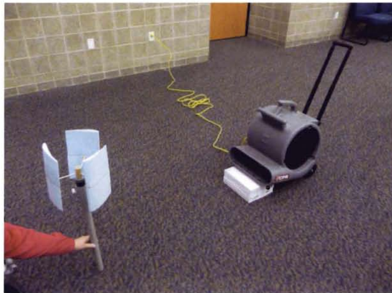
Figure 15: Testing arrangement of small wind turbine and carpet fan.
