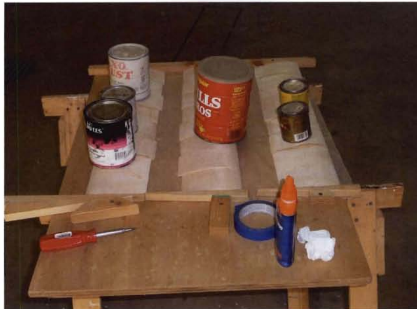
Figure 12: An early attempt to build an S1210 airfoil. (Courtesy of author)
