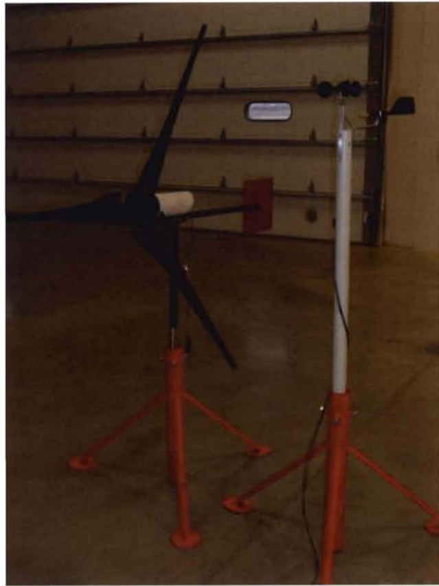
Figure 11: The 1.50 m 2 research HAWT with Windworks Anemometer. (Courtesy of author)
