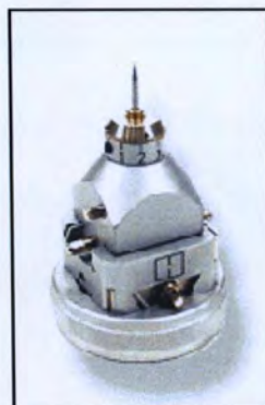
Figure 13. Representative examples of a (A) crystal mounted on a glass fiber and (B) goniometer head for diffraction studies.
