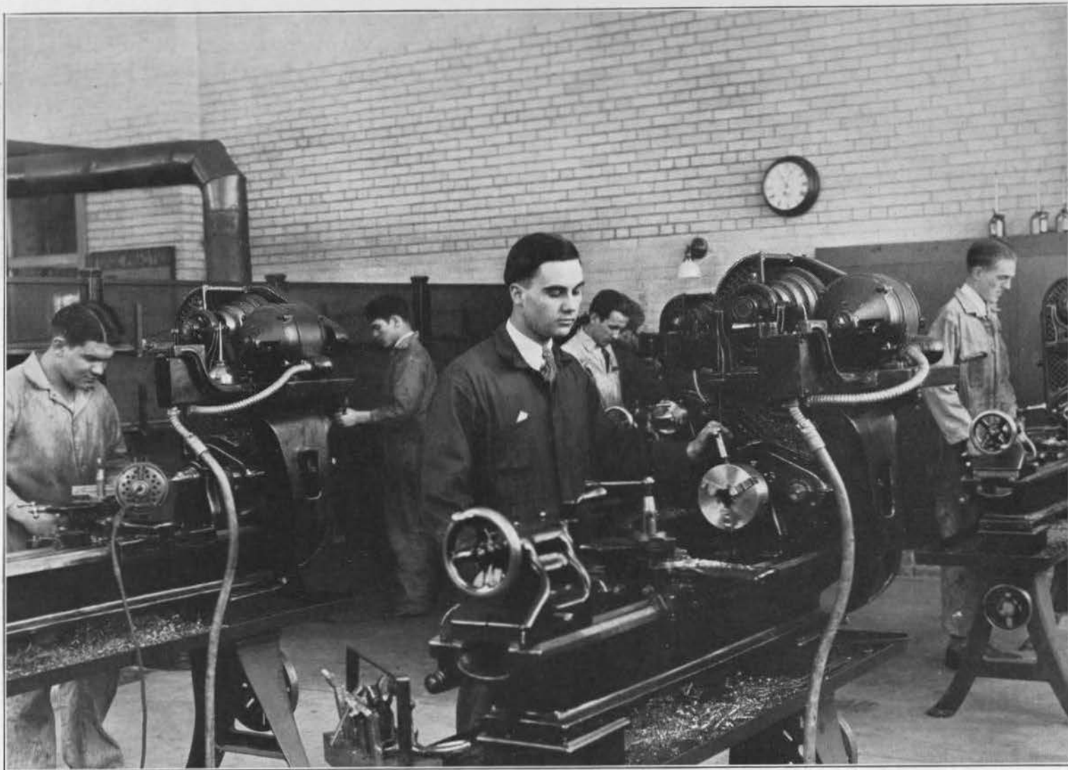
A Battery of Fully Equipped Individual Motor Drive South Bend Lathes Occupy a Portion of the Large General Metal Shop
