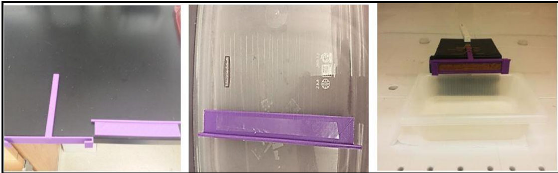
Figure 12 Mass production of nanoendoscopes. (a) A 3-D printed cassette for loading fibers and holder. (b) Multiple (25) fibers loaded onto the cassette. (c) Holder with cassette inserted into HF for fabrication of nanoendoscopes. The process is timed after insertion of cassette holder into HF.
